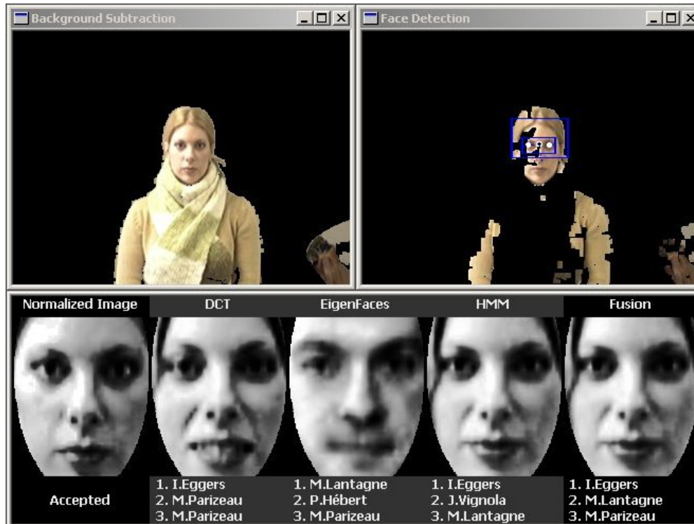
Figure 8: Multi-classifier prototype for face recognition. While the upper-left window represents the background subtraction results, the face detection process is illustrated in the upper-right window. After normalization, the face is presented to several classifiers (i.e. 3 in this example) and results are shown in the bottom window.
