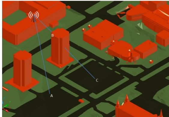
Fig. 1. Direct visibility between an observer and a target, point A is visible while point C is invisible because its line-of-sight is concealed at point B.
