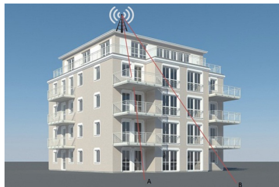
Fig. 7. The impact of completeness on the line-of-sight; Point B is visible but point A is invisible because of the presence of balconies in the building representation
