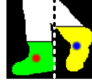
Figure 5. Aggregation of foreground pixels of each leg region (from bottom) until 25% of the number of foreground pixels in the legs region is reached. The mass center of the aggregated pixels is then computed to define a foot position.
