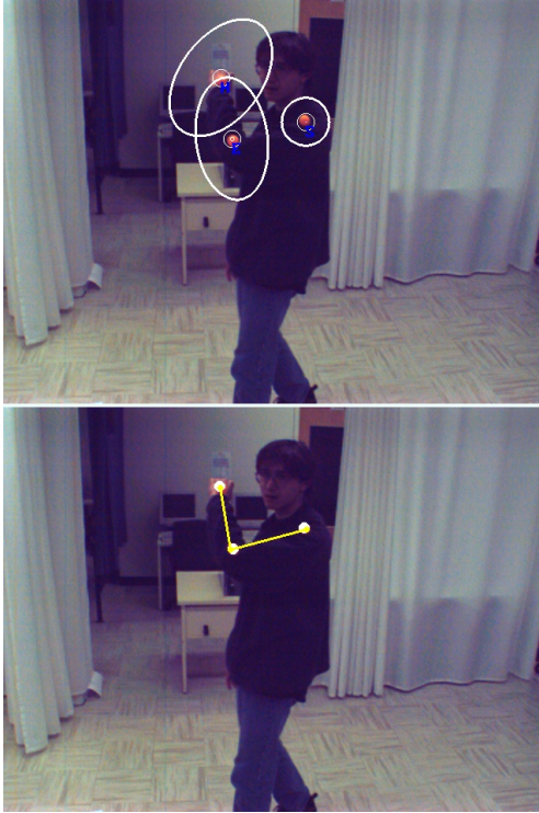
Figure 4: Selected tracking result in the arm sequence. Top: predicted position and size for all markers. Bottom: recovered 3D skeletal model projected in the input image.
