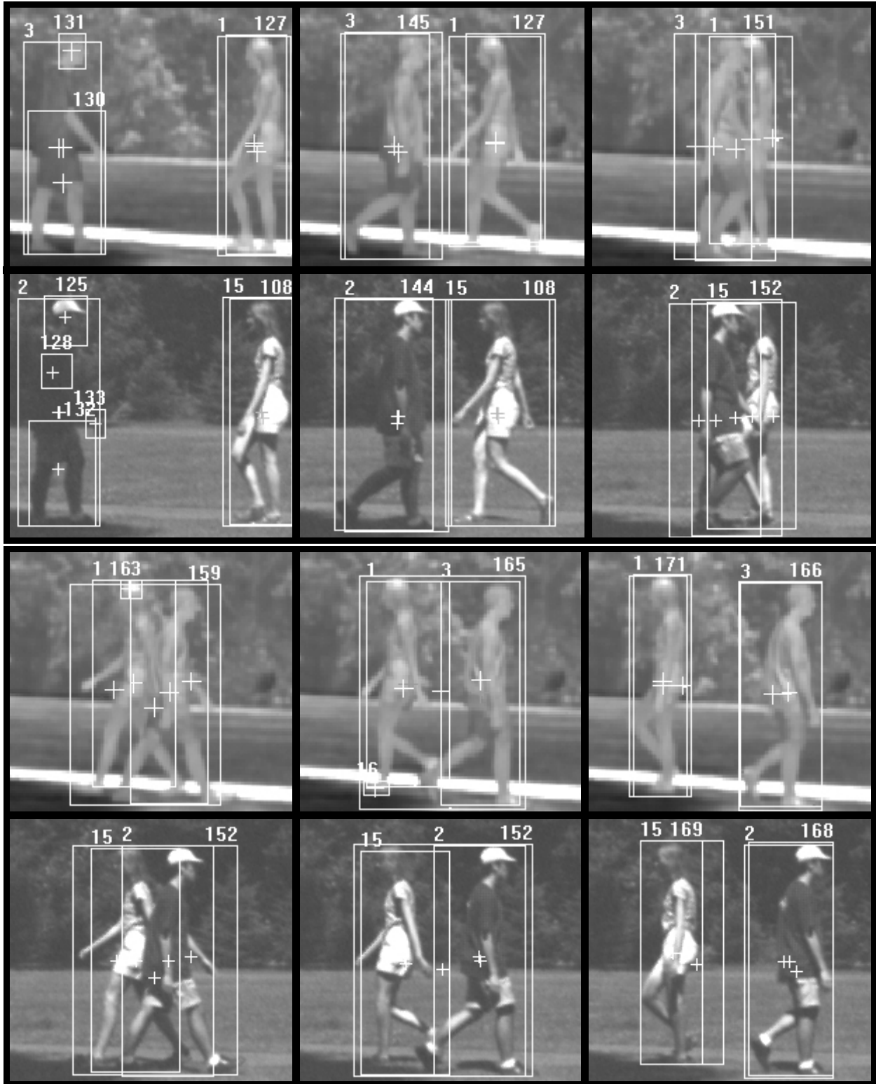
Figure 8: Outdoor scene showing two pedestrians tracked in infrared (upper sequence) and visible (lower sequence) for six snapshots. The labels 1 and 3 represent the two predicted area of the pedestrian in the infrared images and the labels 2 and 15 represent the two predicted areas of the pedestrian in the visible images. The other labels represent the blobs detected by the background subtraction algorithm.
